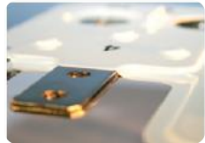
Extra cross-section for localized ampacity reinforcement
